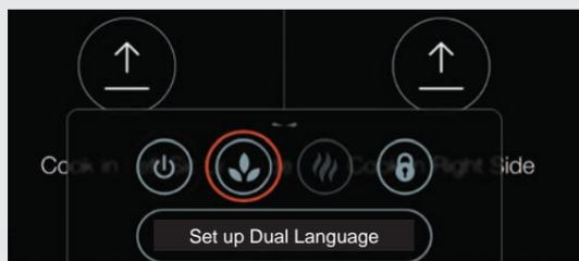
• Swipe up to reveal the quick action dock then tap the ECO mode button. Scan the QR code in the upper right corner to view videos of these procedures and more.
